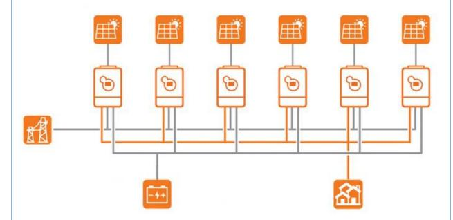
Supports up to 6 devices of the same model connected in parallel (forming a single-phase,split-phase,three-phase electrical system)
