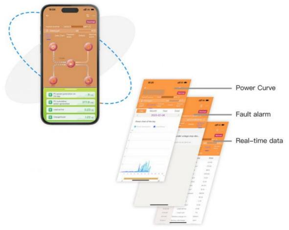
Connection of the specified type of external module (optional) via the dedicated data interface on the inverter, the user can view the inverter's power generation curve and parameters in real time on a mobile app and receive alerts when the inverter is faulty.
